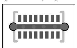
Figure 3 - Recommended Layout Using Ground Vias
